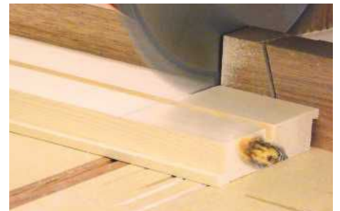
▲ Pic.12 The trenches can be cut by various methods, a radial arm saw being the quickest
